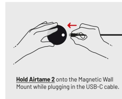
**Hold Airtame 2** onto the Magnetic Wall Mount while plugging in the USB-C cable.
