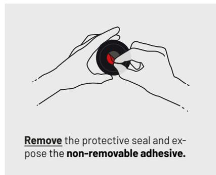
**Remove** the protective seal and expose the **non-removable adhesive**.
