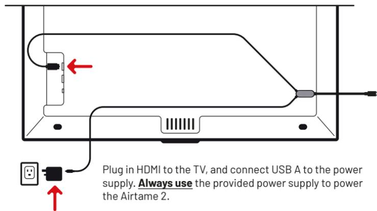
Plug in HDMI to the TV, and connect USB A to the power supply. **Always use** the provided power supply to power the Airtame 2.
